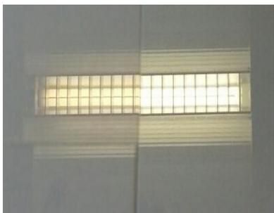
Fig 2 Reflection from light fitting—left side AR coated
