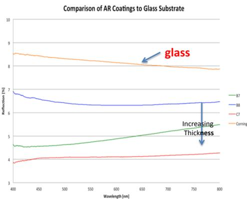
Fig 2 reflection AR on Glass increasing with AR film thickness
