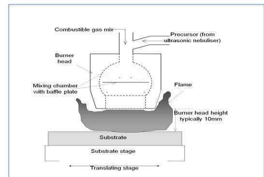
Fig 4 Schematic of FACVD operation
