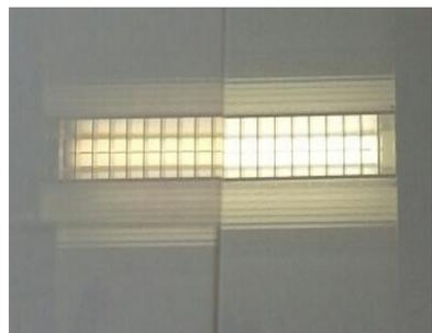
Fig 3 Refl. of light fitting – left side AR coated
